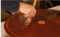
**Two sealcoats.** Working with the grain (top), apply a coat of lacquer sanding sealer using either a conventional flat brush or a mop brush, which can hold more finish. Wait an hour, then apply a second coat, but this time go across the grain (bottom). Let the sealer dry for at least four hours.
