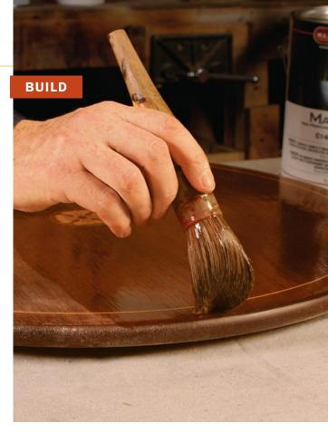
I use M.L. Campbell's Magnasand sealer and Magnamax clear gloss lacquer. Sold by the gallon, they are designed to be brushed or sprayed. Alternatively, Deft, Watco, and Behlen sell quarts of sealers and lacquers. Begin by applying two coats of lacquer sanding sealer, brushing with the grain. Wait one hour, then brush on two more coats across the grain. No sanding is necessary between coats as long as you recoat within four hours.
