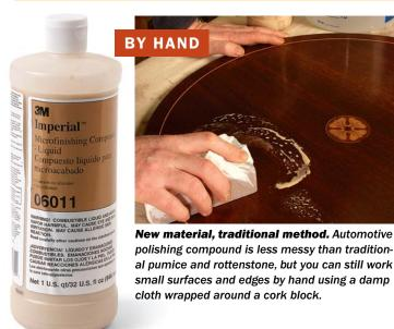
with no lines, wrap a clean cloth around the block. Sprinkle water on the surface, add a small amount of compound to the cloth, and do a final polish with the grain. Finally, use another clean, dry cloth or paper towel to polish off any residue.
